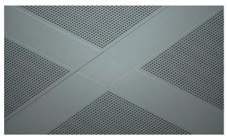
Traditional Two-Way grid systems make the use of trim strips and crossing boxes suspended from threaded rods and hanger brackets. This detail can be replicated by pressing mock crossing details into the C-Profile. Using C-Profiles instead of crossing boxes provides a far more rigid and durable structure. C-Profiles also provide flexibility to avoid costly bridging around ductwork in the void.
