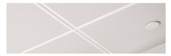
SAS310 is a lay-in tile system which offers the facility to design the metal pan suspended ceiling to suit any building module. The lay-in tiles are suspended from an exposed modular top hat or tee bar grid. SAS310 grid is typically specified as twoway, however one-way options are available on request.
