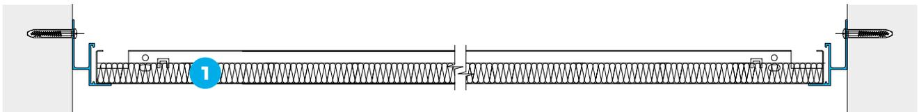
Suspended between walls using perimeter trims.
