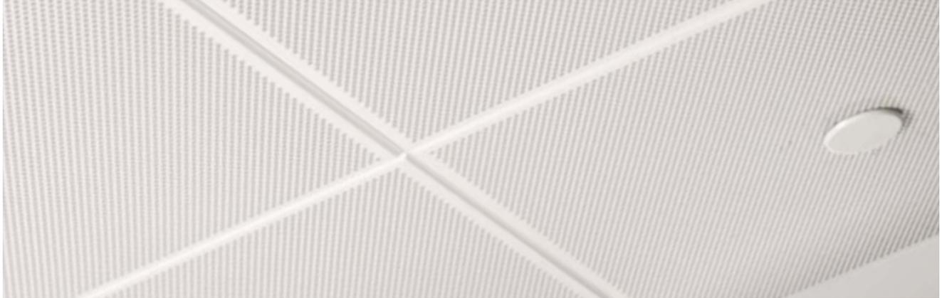
SAS310 is a lay-in tile system which offers the facility to design the metal pan suspended ceiling to suit any building module. The lay-in tiles are suspended from an exposed modular top hat or tee bar grid. SAS310 grid is typically specified as two-way, however one-way options are available on request.
